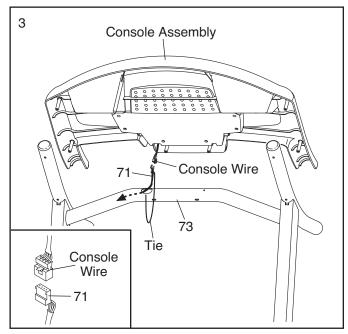
Attach the console assembly to the Uprights (73) and the Handrails (69) with six M4.2 x 19mm Screws (3). Be careful not to pinch the wires.
